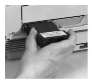
3. Secure the OkiLAN 6010e with the wire clips on the printer's connector.
